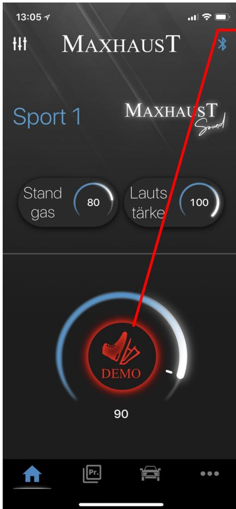
If the DEMO mode is active, you can operate the system regardless of whether the engine is running
