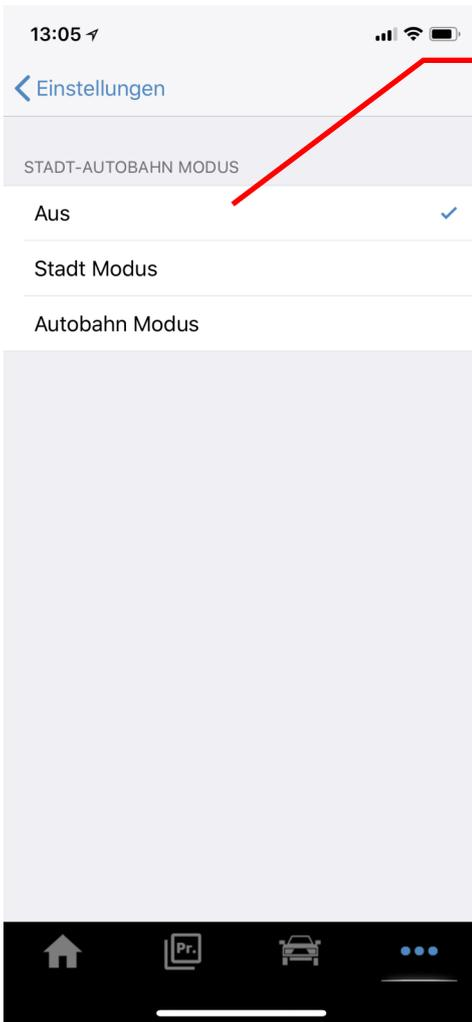
The city-highway mode switches the system OFF and ON again at defined speeds.
